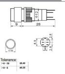
Recommended hole size for installation: Ø12mm
