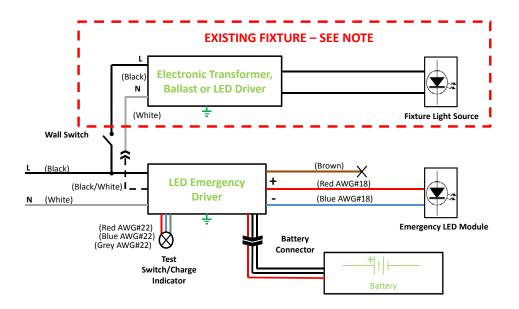
**NOTE:** Existing fixture and light source can be LED, fluorescent, halogen, HID or LED tube.
