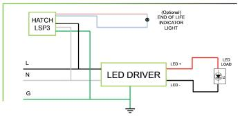
**EOL Indicator:** When illuminated, LSP3 is working correctly. When the indicator goes out, LSP3 needs to be replaced as soon as possible.
