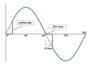
In forward phase dimming, After current crosses zero, the **TRIAC** component in the circuit turns off until voltage is high enough to turn it back on. This type of dimming produces an inrush current so the installer will need to calculate how many dimmers can be installed on the same circuit. This type of dimmer has a very high install base, it's very inexpensive, and easy to install with one wire.
