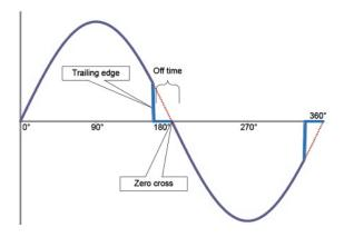
Reverse phase dimming often uses an electronic low voltage (ELV) dimmer to sense when the waveform is approaching zero then triggers the off time. It's a very stable dimming type with low inrush current and compliments LED loads very well. This type of dimmer requires a neutral wire in the junction box.
