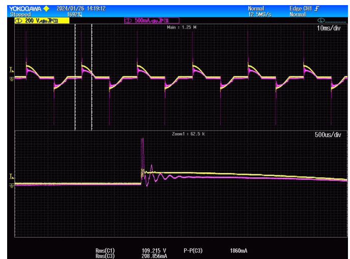
Figure 3 LED Driver Inrush Current on Triac Dimmer
