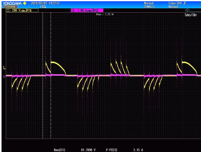
Figure 4 Triac Dimmer Holding Current
